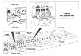
Fig. 1 Layout of ZEBRA - a 300 mA 10 MeV proton linac.
