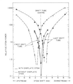
Fig. 6 Stem current versus drift tube support.
