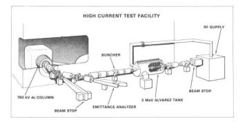
Fig. 7 Schematic of the High Current Test Facility.
