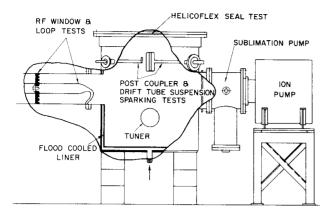
Fig. 8 Schematic of the resonant load facility.
