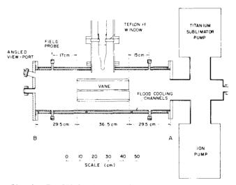
Fig. 4 The RFO Sparker experiment.
