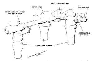
Fig. 3 Injector test experiment for injector development.
