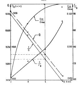
Fig. 2. Cell characteristics versus iris thickness e
