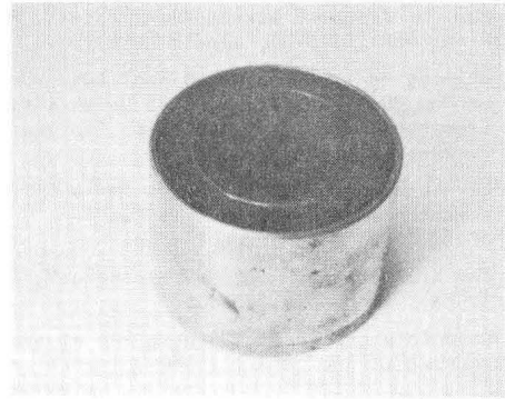
Fig.8 Adjustable gradient samarium-cobalt quadrupole lens developed in IHEP
