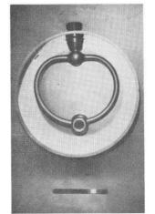
Fig. 10. Low beta lead-plated splitring resonator of the Caltech-Stony Brook design<sup>11</sup>.
