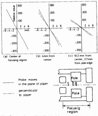
Fig. 7 Focusing radial field. (a) Center of the focusing region. (b) 4 mm from the center. (c) 10.2 mm from the center. Longitudinal length of the focusing electrode is 13 mm and distance between the electrode chips is 20 mm. Dependence of the focusing field on the azimuthal position is clearly seen.
