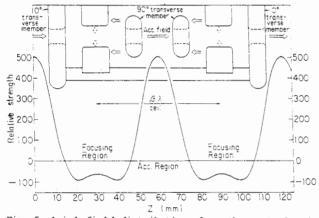
Fig. 5 Axial field distribution along the central axis of the Type 2 structure.
