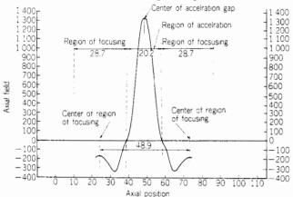
Fig. 4 Axial field distribution along the central axis of the Type 1 structure.
