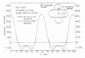
Fig.6 Axial field distribution along lines 3 mm off axis of the Type 2. In the focusing region, the distribution changes according to the azimuthal positions of the lines.
