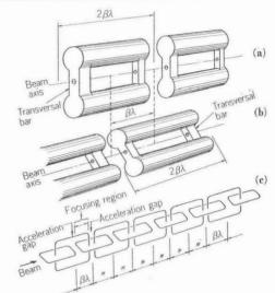
Fig. 1 How to combine electrodes to form a chain-like accelerating structure. (b) is rotated around the beam axis by 90 degrees compared to (a). (c) shows interlacing of (a) and (b).
