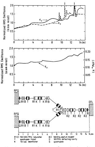
Fig. 2: rms emittances along the funneling line
