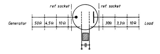
Fig. 2 Equivalent circuit of the amplifier
