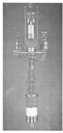
35 MW Pulse-Klystron YK 1600
