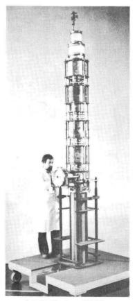
1,5 MW Klystron V107SK
