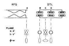
Fig. 1. Schematic representation of matched phase spaces at end of RFQ (A), and at midquad (B and D) and gap (C) in DTL.
