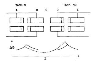
Fig. 2. Longitudinal matching between DTL tanks. Solid lines show normal drift tubes and phase profiles. Dashed lines show modified drift tubes and resulting change in phase profile.
