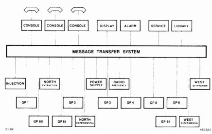
Fig. 2. Single layer architecture at the SPS 1976.
