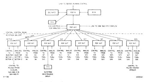
Fig. 1. Master/slave architecture at SLAC 1974.
