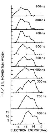
Fig. 5 Energy spectra of an accelerated beam observed every 100 nsec.
