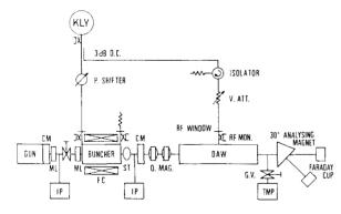
Fig. 4. Experimental setup for the beam test of the accelerating tube.
