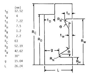
Fig. 3. Parameters of the DAW accelerating structure.
