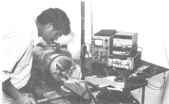
Fig. 5. Tuning an RTM half-cell on a lathe using electronic measurement methods.
