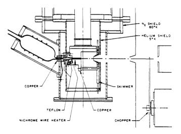
Fig. 3. RF dissociator and accommodator shown mounted to the base of the LHe cryostat. The RGA (not shown) is to the right.
