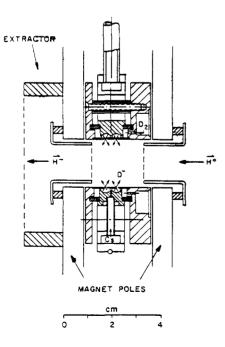
Fig. 5. Schematic of the ring-magnetron ionizer.
