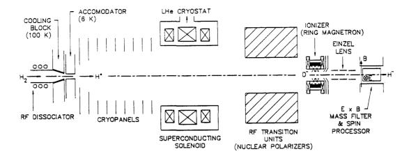
Fig. 2. Layout of the proposed milliampere H source.
