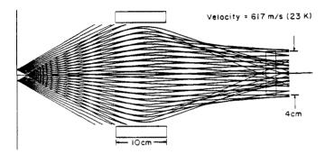
Fig. 4. Output of the track-tracing program for  $B_0 \sim 5T$  and R = 5 cm at the mid-plane of the solenoid.
