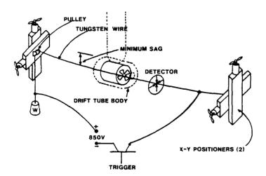
Fig. 1. Alignment of drift-tube quadrupoles using pulsed wire.
