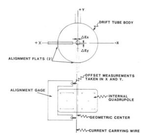
Fig. 4. Alignment jig for measuring magnetic-axis offset.
