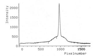
Fig. 3: The beam profile of a 60 keV H<sup>+</sup> and H<sup>+</sup> beam of 17 mA with an integration time of 200 msec (without image amplifier)
