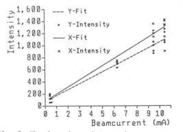
Fig. 5: The dependence between beam current and video signal.
