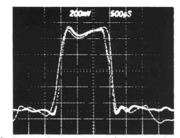
Fig. 9: Input and reconstructed (dotted line) pulse for a complete 200 MHz period
