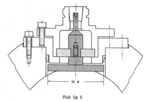
Fig. 7: Schematic drawing of pick up type II
