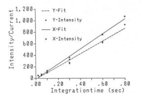
Fig. 4: The dependence between integration time and normalized video signal.
