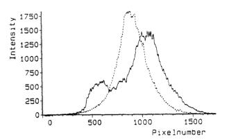
Fig. 1: The horizontal and vertical beam profile of a 860 keV H<sup>+</sup> beam of 15 μA, with an integration time of 10 sec (corrected for background)
