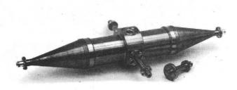
Fig. 6: Photograph of the capacitive pick up probes inserted in the center of the 50 & -coaxial test facility
