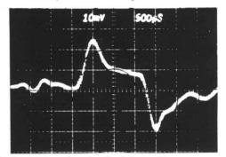
Fig. 10: Response signal of pick up II
