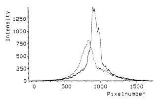
Fig. 2: The horizontal and vertical beam profile of a 860 keV proton beam of 10.5 mA with an integration time of 300 msec (corrected for background)
