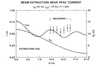
Figure 7: The rms radius calculated with DYNADISC. The solid circles with the error bars are the experimental envelope measurements with the radiochromic foils.
