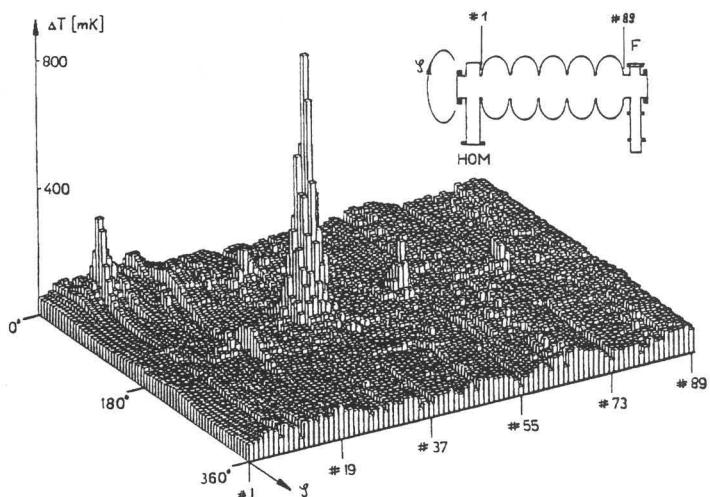
FIGURE 3. Temperature map of a superconducting CEBAF cavity at  $E_{acc} = 5.6$  MV/m, taken with a thermometry system consisting of a rotating array of 89 temperature sensors. This system scans the cavity surface for enhanced losses and permits guided repair to be performed.<sup>14</sup>
