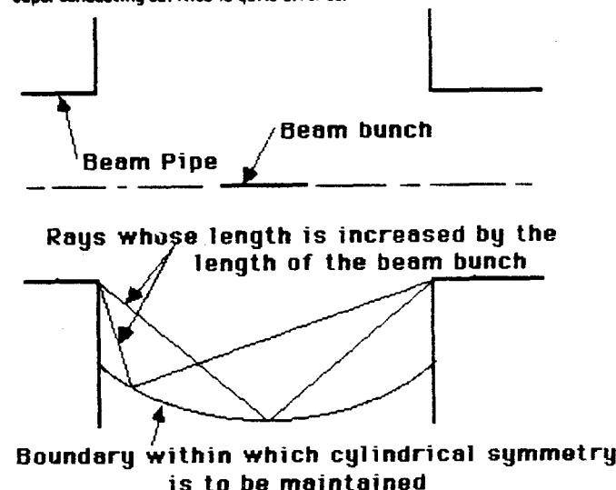
FIGURE 2. LIGHT CONE SYMMETRY.
