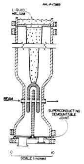
Fig. 1 Cross Section of a 48.5 MHz, 10 cm interdigital resonator. A coaxial, tapered quarter-wave line is terminated in a four-gap interdigital capacitive load. The resonant cavity can accelerate particle with velocities below .01c and has an active length of 10 cm.
