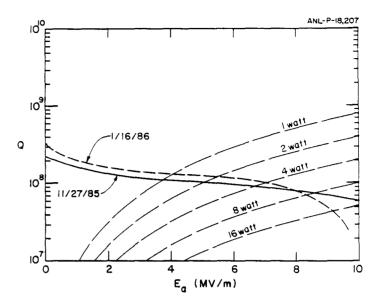
Fig. 3 Resonator Q vs effective accelerating gradient E measured at 4.2 K for the superconducting 10 cm interdigital structure. Also shown is the rf power loss at various field levels.
