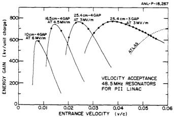
Fig. 2 Voltage gain per unit charge per resonator for four different resonator geometries which can form an injector linac. The discrete points show single-resonator velocity increments for a 20+ uranium beam.
