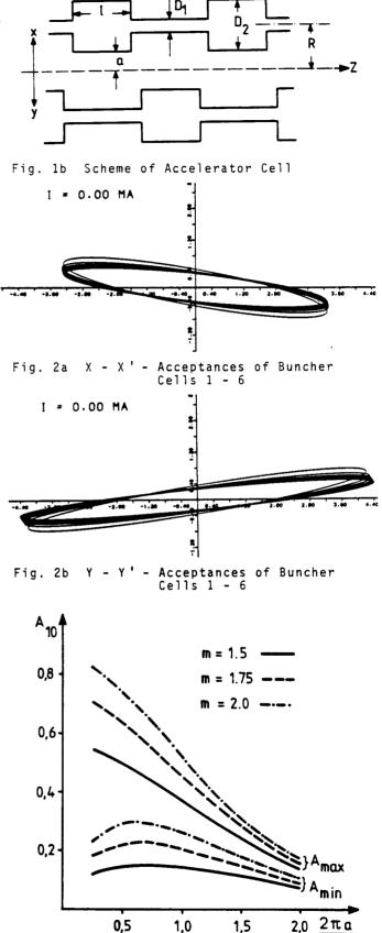
Fig. 3 Range of Acceleration Rate A10 versus normalized Aperture at different Modulation
