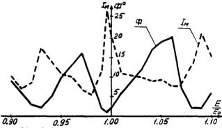
Fig.6 The dependances of a phase length of a bunch  $\Phi$  at 0.5 level and maximum of bunch density distribution  $I_M$  on the amplitude of rf field.
