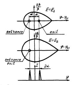
Fig.7 Qualitive explanation of the rf phase setting method.
