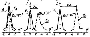
Fig.8 Bunch density distributions and relative phase positions of bunchs for  $E_1 = 0.955E_0$ ,  $E_2 = 1.035E_0$  and different  $\Psi_{en}$ .
