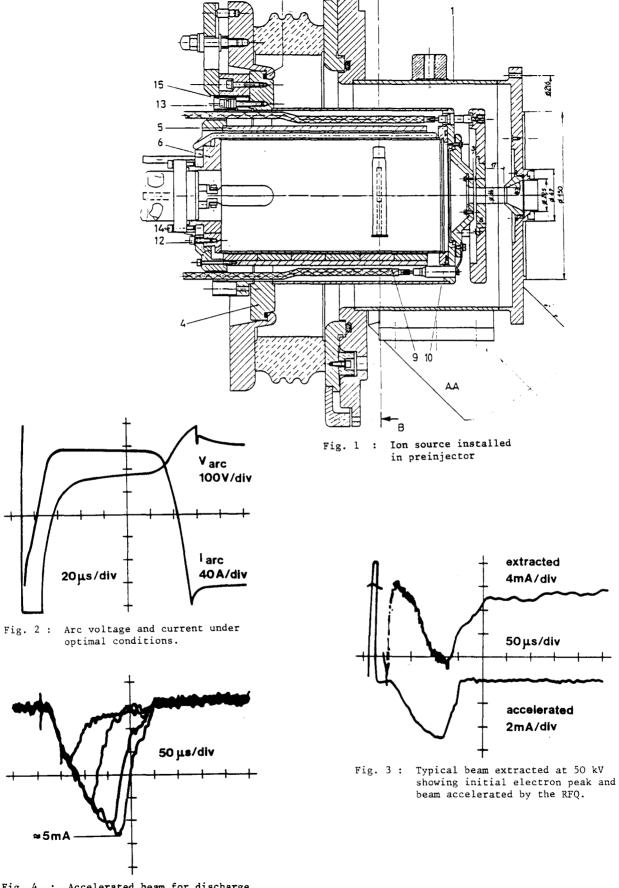
Fig. 4 : Accelerated beam for discharge lengths of 50, 100, 150, 175 uS. Source parameters constant.
