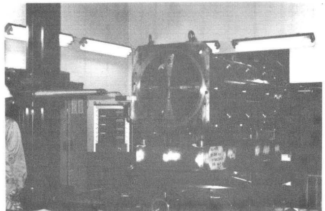
Fig.1. Inspection of the vane alignment.
