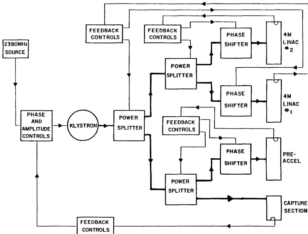
Figure 1. Block diagram of RTM RF control system.
