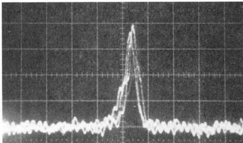
Figure 3. Wirescanner output X (energy analyzed) plane. Horizontal scale is 2.15 mm per division, or 50 keV. Vertical scale is current, in arbitrary units.
