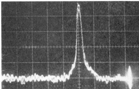
Figure 4. Wirescanner output Y (not energy analyzed) plane.
