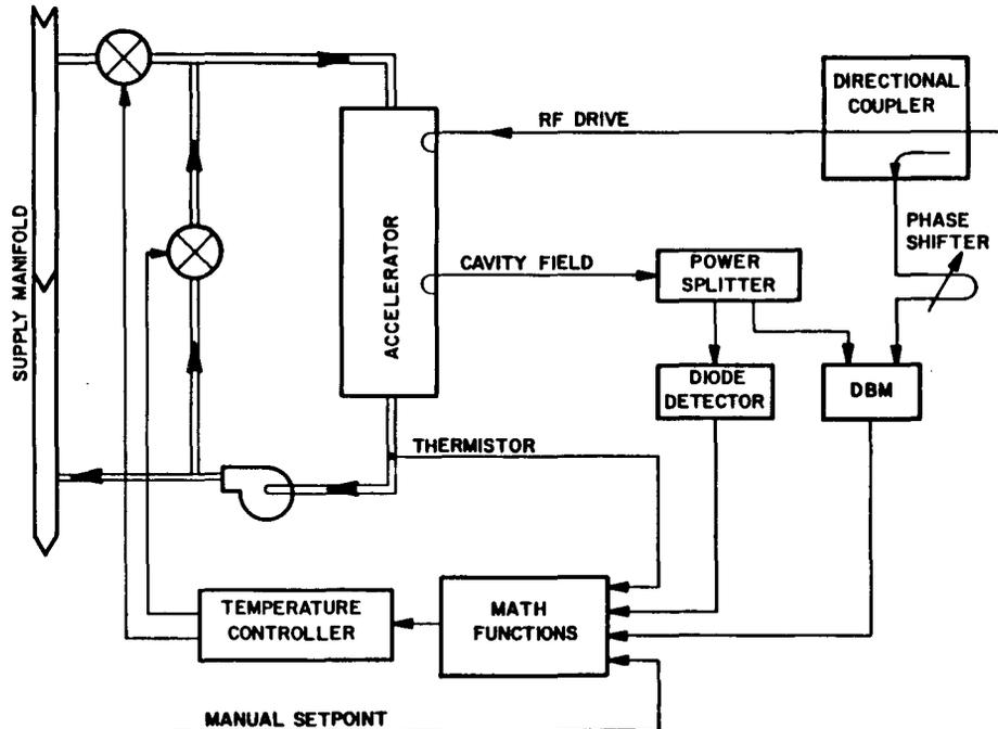
Figure 2. Block diagram of RF resonance control system.
