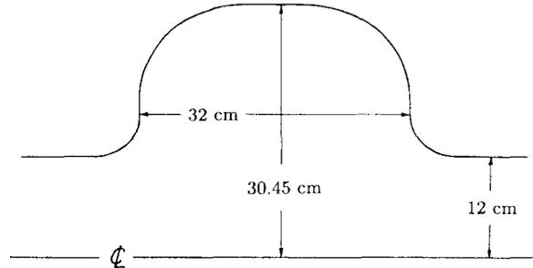
Fig. 7. The profile of the elliptical cavity.
