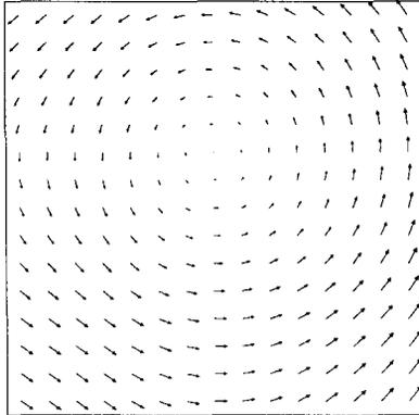
Fig. 5. A close-up of the magnetic field in Fig. 4 near the cavity center shows the field asymmetry. The cavity center is at the center of the picture.
