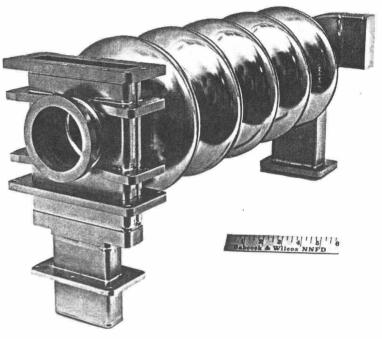
**CEBAF** Cavity Fabricated by B&W
