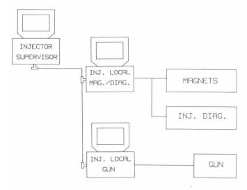
Figure 4 Injector Distributed Architecture
