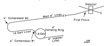
Fig. 1. Schematic of a Next Linear Collider
