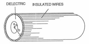
Figure 5: Deflection mode damping dielectric WF tube
