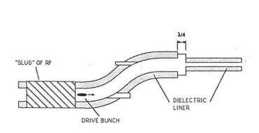
Figure 6: Schematic CWFA section
