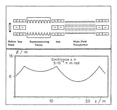
Figure 2: A RWT based cell of a high energy linac.
