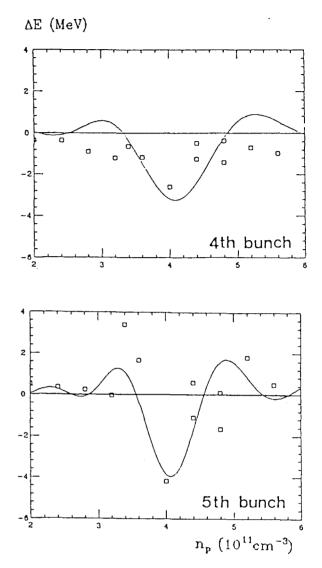
Figure 3: Observed energy shifts of the 4th and 5th bunches as functions of plasma density in the KEK PWFA experiment.
