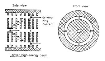
Figure 1: The wake field transformer.
