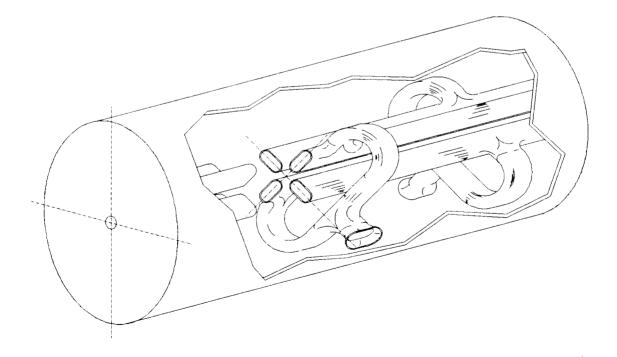
Fig. 1 Conceptual design of a low-frequency SCRFQ accelerator structure.
