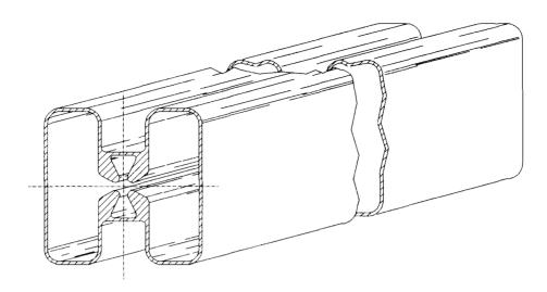
Fig. 2 Conceptual design of a high-frequency SCRFQ accelerator structure.
