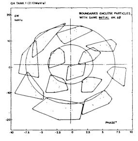
Figure 1: Coupling from Transverse to Longitudinal Phase Plane
