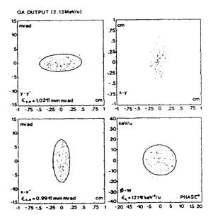
Figure 2: Phase Plane Projections at 2.13 MeV/u
