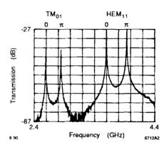
Figure 2. Single-cavity resonances excited through probes C or D so that they cannot couple through the ridged waveguides.
