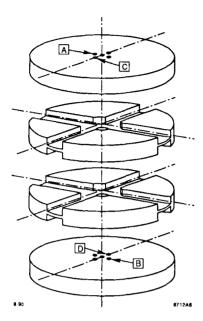
Figure 6. Azimuthal waveguide structure.
