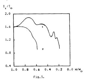
The higher is the value of  $\mathbf{W}_{o}$ , the higher are both the efficiency and the output power of the system.
