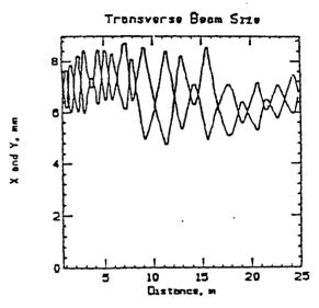
Figure 5 Beam envelope for positron accelerating sections
