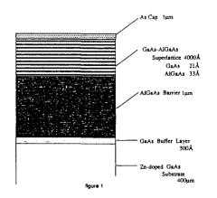
50%) electrons coming from the GaAs substrate. Then, GaAs-AlGaAs SL layers were grown. The layer thickness of GaAs (AlGaAs) was 21Å(33Å), respectively. The final layer of the SL was GaAs. The surface of the SL is covered by Arsenic for protection against atmosphere. Band structures of the SL calculated by a method in ref.7 are summarized in figure 2.
