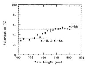
corresponds 50meV) agrees with the calculated energy gap between the top of heavy hole band and the top of the light hole band (43.4 meV) as shown in figure 2. There are no measured points below 700nm of wavelength because our laser dose not work there.
