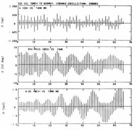
Fig. 5. Beam size of singlet lattice with a combination of random errors within  $\pm$  -- 0.004" quad displacements, 0.010" tank displacements, 2% quad gradient errors and 1° phase errors.
