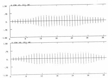
Figure 3. X and Y beam profile through the HESQ.
