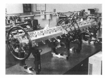
Figure 1 - Radio Frequency Quadrupole
