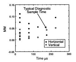
Fig. 6. Horizontal and vertical MM (IMS output beam) versus time within the macropulse. Maximum MMs are ~0.1 in x and ~0.05 in y indicating no significant changes in the CS parameters during the macropulse.
