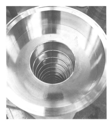
Figure 4. Linac cell stack.
