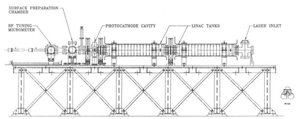
Figure 2. AWA photocathode gun and preaccelerator.
