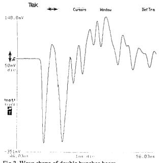
Fig 3 Wave shape of double bunches beam, Anode voltage: 170 kV, Heater voltage: 6.0 V, Net drive voltage: 260 V, Vacuum 2x10<sup>-8</sup> Torr
