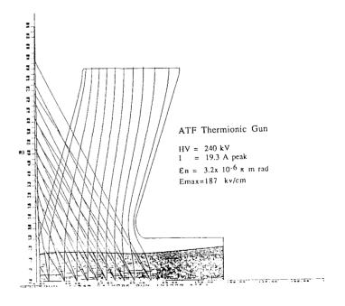
Fig.1 Beam trajectory
