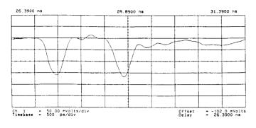
Fig.2 Output of the double-pulse generator (100V/div, 500ps/div)
