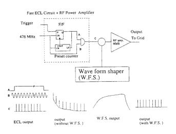
Fig 4 Schematic drawing of multi-pulse generator.
