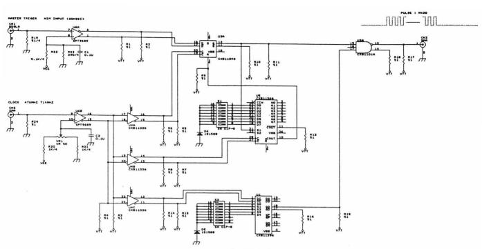
Fig.5 Circuit diagram of the fast ECL of multi--pulse generator
