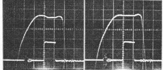
(1)ALC only (2)ALC+Compensation Fig.5 Tank field and pulse beam upper : Tank field (6.7%/div) lower : pulse beam (2mA/div)
