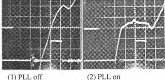
(2) PLL on Fig.6 Effect of PLL upper : phase (2.5deg/ div) lower : pulse beam (2mA/div)
