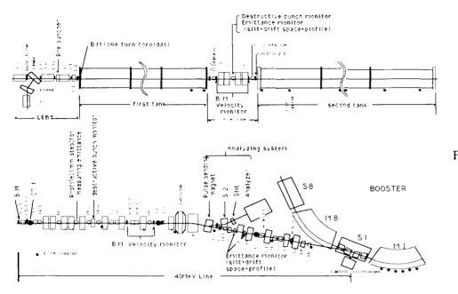
Fig.2 Layout of the KEK Proton Linac and the Beam Lines
