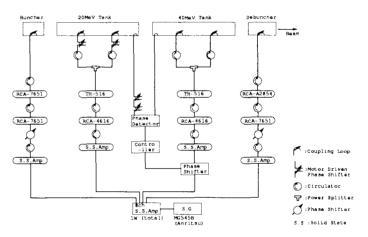
Fig.1 Block diagram of present RF system for the KEK 40MeV Proton Linac
