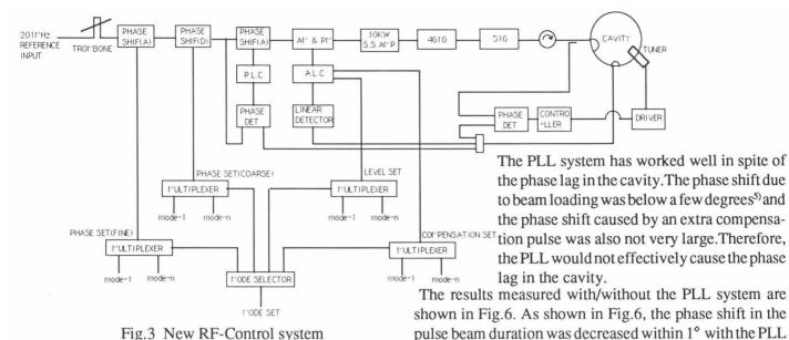
Fig.3 New RF-Control system
