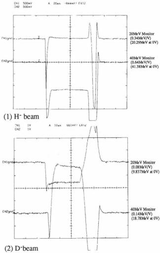
Fig.4 The measured results using Velocity Monitors (1) H<sup>-</sup> beam, (2) D<sup>-</sup>beam
