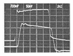
Fig.3 Pulse responce of one turn toroid (upper: input, lower: output)
