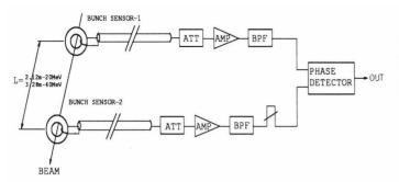
Fig.1 Block diagram of velocity monitor
