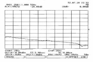
Fig.2 Frequency characteristics of one turn toroid
