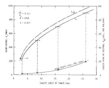
Figure 1. Traveling Wave Structure Input Power and Peak RF Voltage versus Beam Energy and Ring Orbit Loss.
