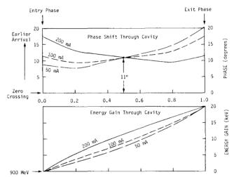
Fig. 3. RF Cavity Phase Orbit and Energy Gain <u>vs</u> Distance Along Structure for  $P_0=26kW$  and  $V_0=900MeV$  (0.11%  $\Delta V/V$ ).
