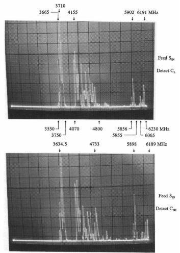
Figure 5. HOM Extraction Circuit Output Signals for a 2 to 6 GHz Swept Excitation of the TW Structure.
