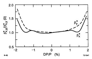
Fig. 5. Energy passband of the DLC Final Focus.
