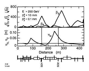
Fig. 6. Optics of the JLC Final Focus.
