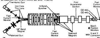
Figure 1. SLC injector beam line up to the fast current monitor at 40 MeV.
