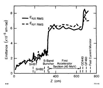
Fig. 5. Normalized emittance from the GUN to the fast current monitor at 40 MeV.
