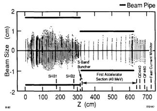
Fig. 3. Beam radial profile from t he gun to the fast current monitor at 40 MeV.
