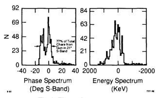
Fig. 4. Electron beam parameters at the fast current monitor at 40 MeV.
