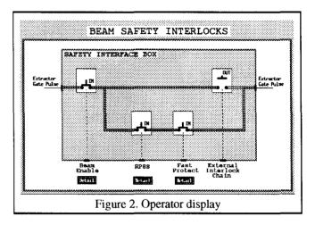
The screen shows a partial schematic of the wiring of the extractor pulse from the timing system to the injector. The Run Permit system operates one of the switches which interrupts the pulse (the one labelled Beam Enable). If Run Permit is presently enabling the injector, this screen will show the switch closed, as in the figure. If Run Permit issues a disable signal, the switch appears open.
