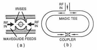
Fig. 1 Schematics of RF power input to coupler.
