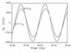
Fig. 7 Amplitude and phase asymmetries in a single input coupler cavity.
