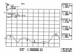
Fig. 6b Cold-test data of VSWR versus frequency.
