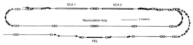
Figure 2. Configuration of Magnetic Elements in the Beam Transport System.
