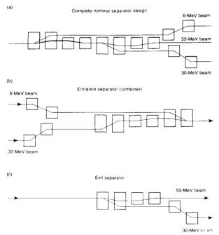
Figure 3. Separator Configurations: (a) Fully Loaded, (b) at Entrance and (c) Exit Ends of SCA.
