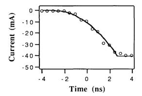
Fig. 7. Leading edge of first waveform in Fig. 5. the solid curve represents theory and the circles experiment.
