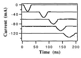
Fig. 2. Beam current waveforms for drift expansion.
