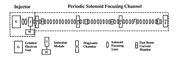
Fig. 1. Experimental configuration.
