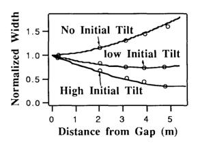
Fig. 4. Normalized bunch width vs. drift distance for parabolic bunches where the solid curves represant theory and the circles experiment.
