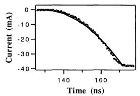
Fig. 8. Leading edge of last waveform in Fig. 5. the solid curve represents theory and the circles experiment.
