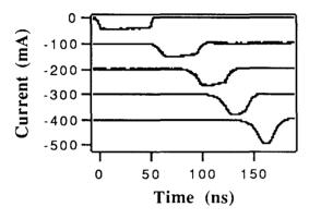
Fig. 6 Beam waveforms for drift compression.
