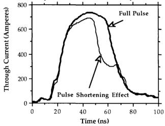
Figure 4. Normal overlaid with shortened pulses.
